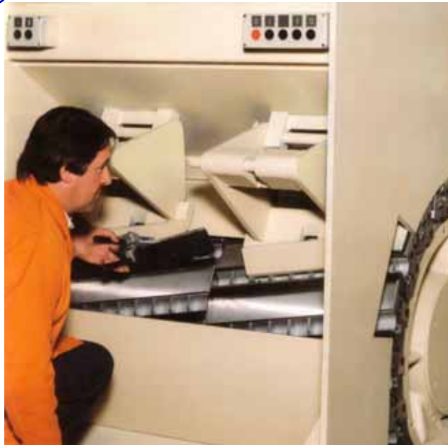
Wedges are pressed down hydraulically
