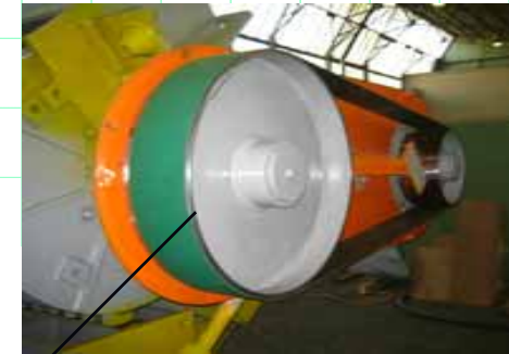
Drive of rotor with flat belt Without cover
