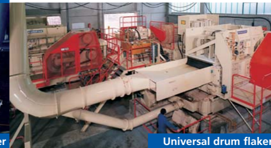
Drum flaker for pre-cut timber
