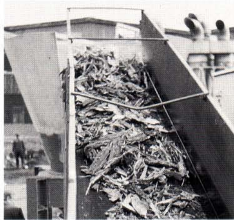
Belt conveyor to the Bark Shredder
